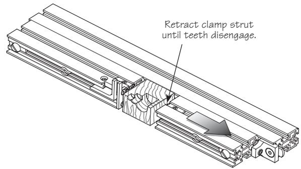
**Figure 28: Retract clamp strut and remove used wood backing block.**
