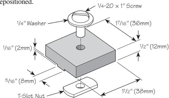
**Figure 32: Typical sled stop.** Dimensions given are maximum.
