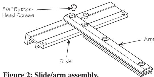
**Figure 2: Slide/arm assembly.**
