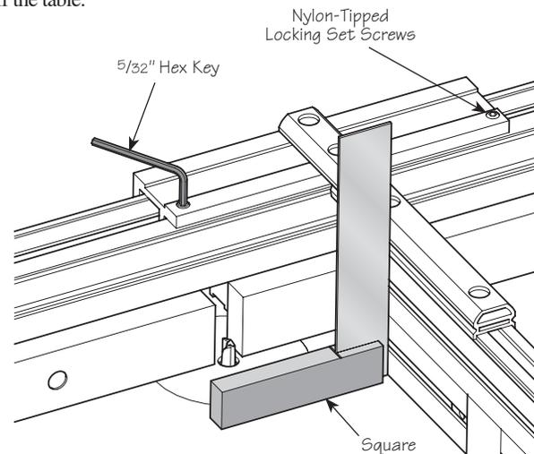
**Figure 4: Perpendicular adjustment.**
