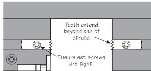
**Figure 29: Ensure teeth extend beyond end of struts.**
