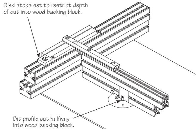
**Figure 20: Set-up for cutting finger joints.**
