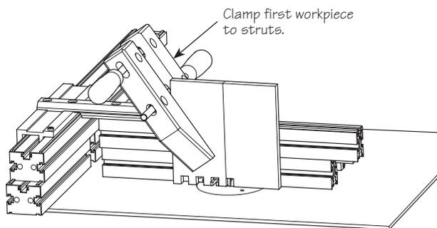
**Figure 23: Cutting finger joints in two pieces.**
