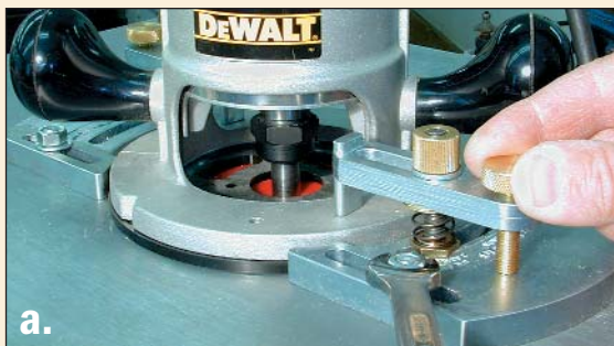
a. A unique, quick-clamp mechanism on the Veritas router table lets you mount or remove the router in seconds.
