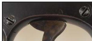
If tip extends beyond edge of head, adjacent area will be marred.
