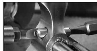
Base Pin Latch Nut requires the correct tool.
